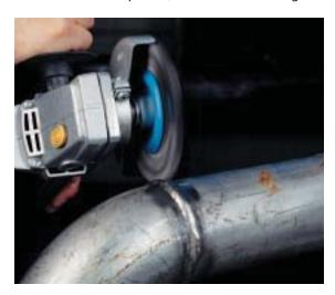
✓ Knot-twisted and double-row brushes are for surface cleaning after welding, to remove scale, spatter, rust and corrosion
